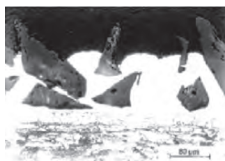
Ni-SiC-Composite Schicht fürs Schleifen
